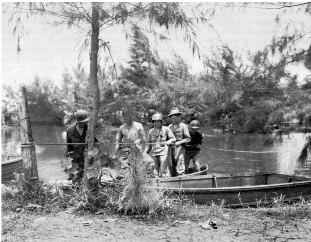
COLLAPSIBLE ASSAULT BOATS being used by 127th Infantrymen to cross the Siwori Creek. Note guide rope across the creek.
